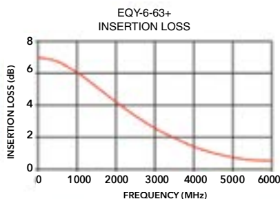
Figure 7: Insertion loss response for EQY-6+ MMIC equalizer with -6 dB slope.
