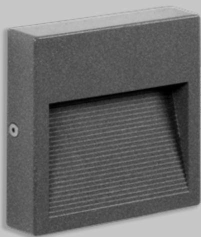
Series of Wall-mounted luminaires made in aluminium alloy (EN AB 44100) with high resistance to oxidation and subjected to a treatment of nanoceramic bonderite that, with the powder coating polyester, guarantees to the product a highly resistant to the atmospheric agents and UV rays, ensuring maximum protection over time.
