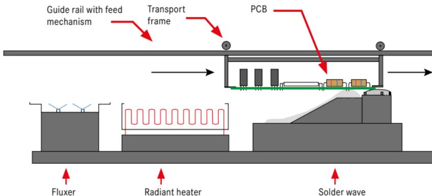
Figure VIII-1: Principle of wave soldering
