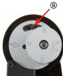
Ⓑ 2. Unlatch the settings dial (pull it out) and then turn it until the desired number is visible in the scale on the back of the crimping tool **Ⓑ**. Release the settings dial; give it a brief turn so that it latches back into place.
