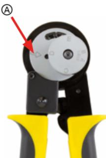
The arrow Ⓜ will indicate the selected marking. The locator will latch back into position when you release it.
