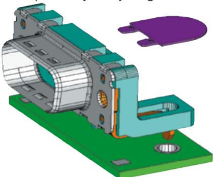
Figure VIII-5: D-sub SMC connector
