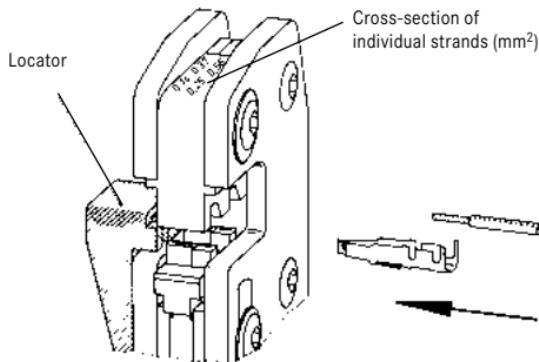
Figure V-15: Feeding of the contact
