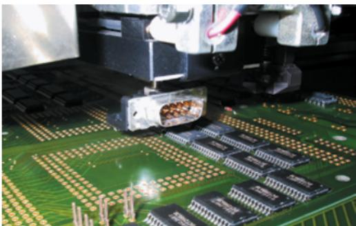
Figure VIII-6: Pick-and-place machine with vacuum pipette and D-Sub
