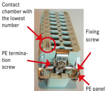
Figure II-1: PE termination for the Han® 16 E insert
