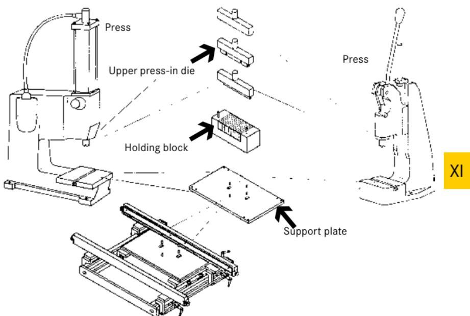
Figure XI-6: Construction of HARTING's modular tool system
