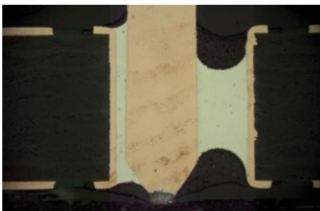
Figure VIII-11: Soldered joint with borderline degree of filling
