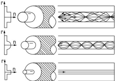
Figure XII-1: Path of the optical refractive index
