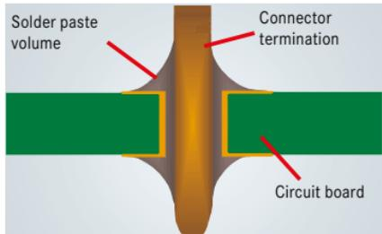
Figure VIII-8: Plated through-hole with connector termination
