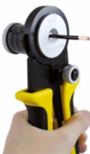
3. Press the crimping tool's handles together in order to crimp the contact. Press the handles closed until they automatically reopen (refer also to the chapter Ratchet lock, p. 83).
