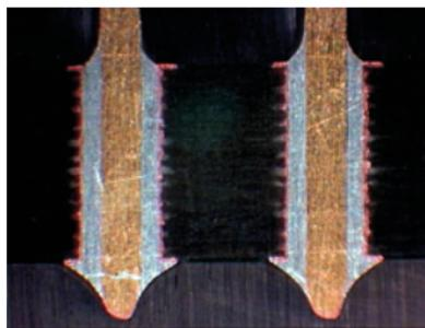
Figure VIII-10: Fault-free soldered joint
