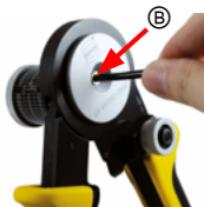
2. Insert a properly stripped wire into the crimp contact Ⓑ.
