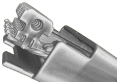
Figure X-19: Micro-section of piercing termination technique
