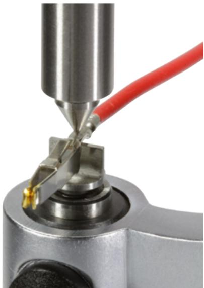
Figure V-10: Detail view of crimp contact
