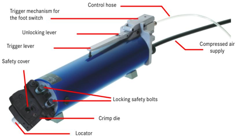
Figure V-20: Overview of HARTING pneumatic crimping tool CP 600
