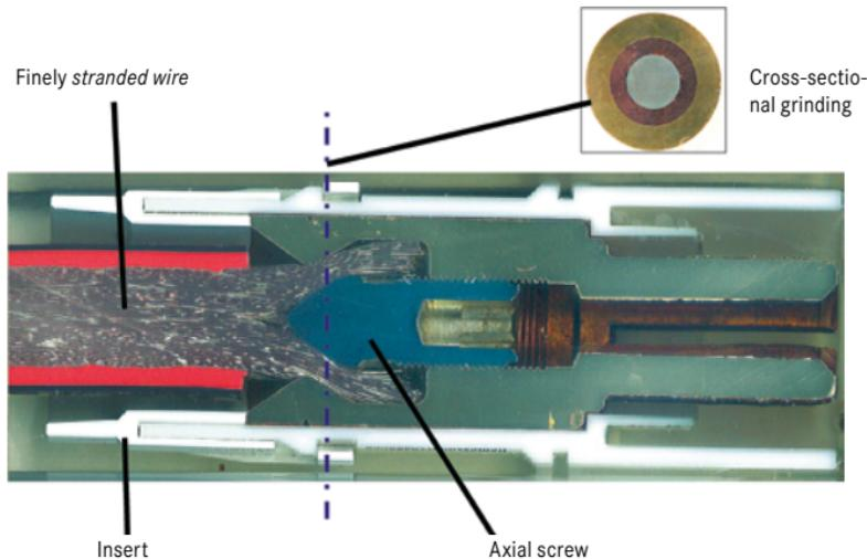
Figure IV-1: Micro-section of axial-screw contact (longitudinal + cross-sectional grinding)
