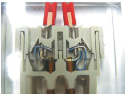
Figure VI-4: Termination with ferrule crimped on
