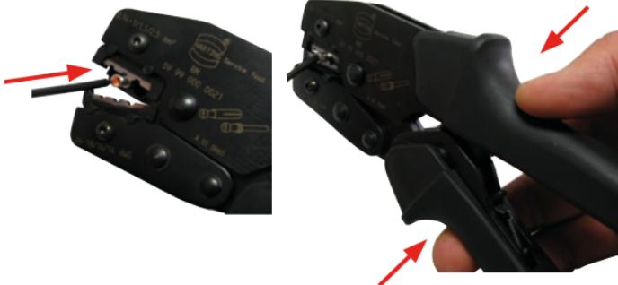
3. Remove the crimped contact
