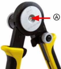
1. Insert the crimp contact into the tool opening Ⓐ. The locator ensures that the crimp contact is automatically positioned in the proper crimping position.
