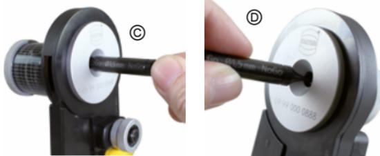
**Your crimping tool must be re-adjusted by a trained technician, if it does not pass this test!**
