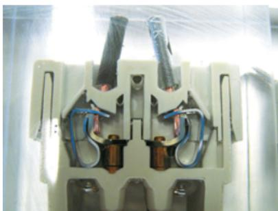
Figure VI-5: Termination with stripped stranded wire
