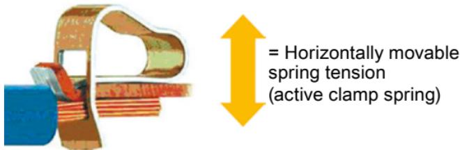
Figure VII-2: Cage-clamp termination
