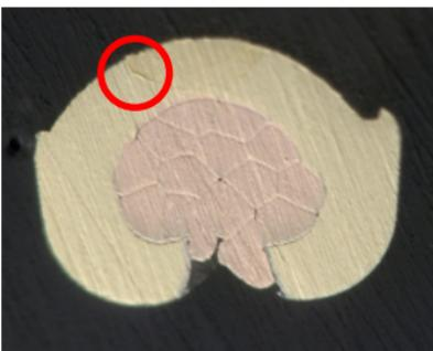
Figure V-6: Micro-section of a defective sample with cracks
