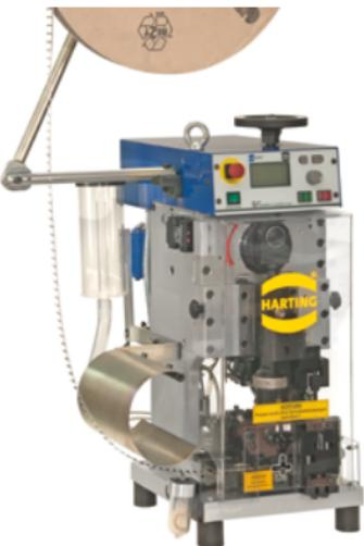
Figure V-18: TYPE BK crimping machine (fully automatic machine)
