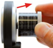
Select the series to be processed – Han D®, Han E®, Han® C or Han-Yellock®. Pull the locator out of the latch and turn it until the required marking is lined up with the contact position.
