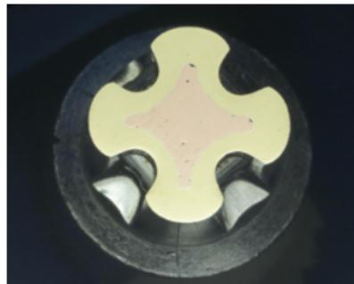
Figure V-1: Micro-section of a flawless sample
