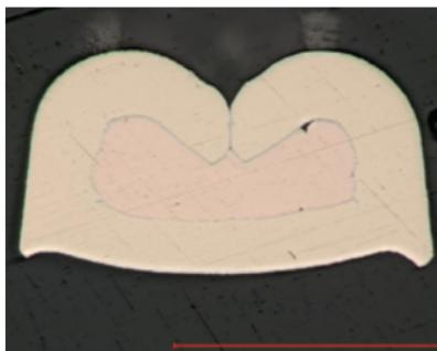
Figure V-5: Micro-section of a flawless sample
